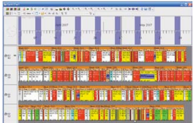
Figure 4: Manual schedule. The color code is: red if the supplied item is below 0 at the time of the event, yellow if it is above maximum, green if it is below minimum, blue if it is below alarm and white if it is within the tunnel. Note that many items are produced when they are red (customer service failure) or yellow (over-stocking).
